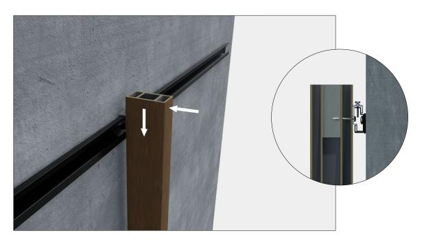
**STEP 4** Install the Brise Soleil using the NV3 clip on the rail.
