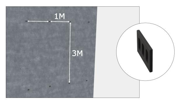
STEP 1 Add a thermal break pad (ref 1157) between the rail and the support. A calculation note with the calculation of wind loads and shear forces is available for each profile.
