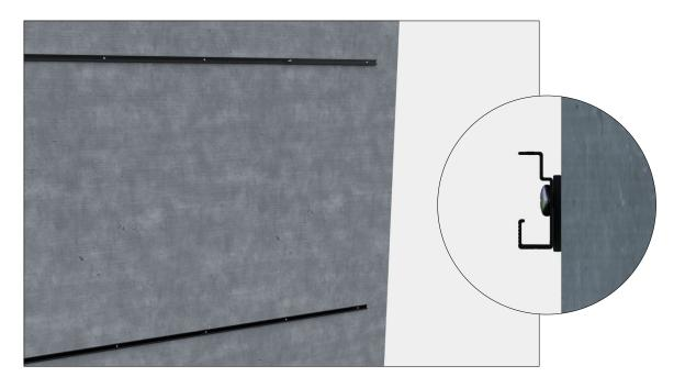
STEP 2 Fix the rail (ref 1156) on the load-bearing wall with fixings suitable for the support.
