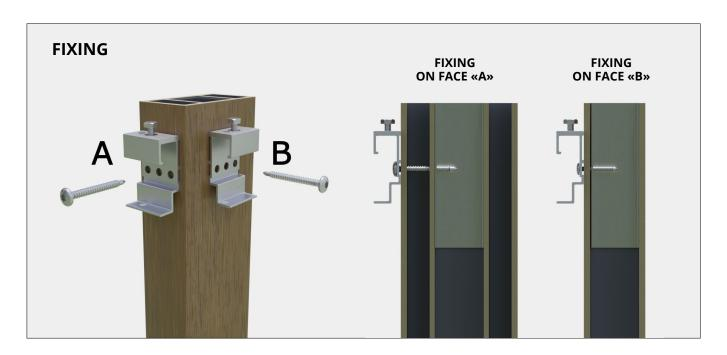
STEP 3 Each Brise Soleil can be installed on 2 different sides (A or B).
