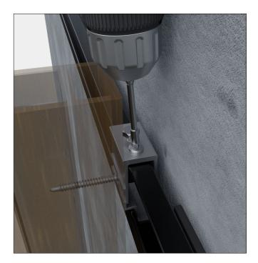
**STEP 5** Adjust the verticality of the Brise Soleil with the M6x20mm adjustment screw. Then screw the NV3 clip onto the rail with a 5.5x32mm screw using a long bit.
