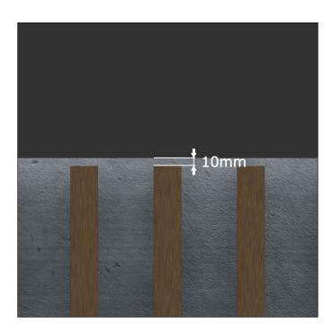
**EXPANSION GAP** Leave a gap of 5mm between 2 ends of Brise Soleil and 10mm between a Brise Soleil and all types of obstacles encountered (carpentry, wall, angle, etc.).
